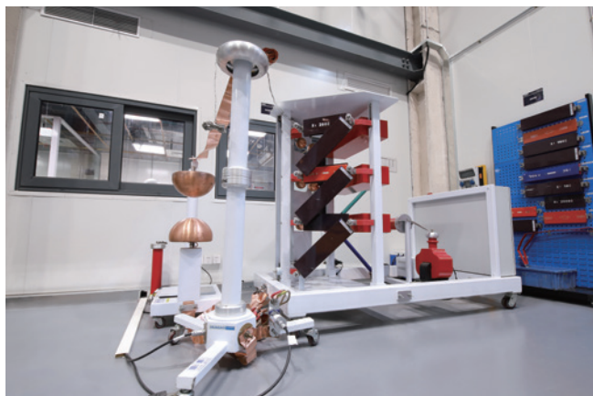
Lightning Impulse test system
